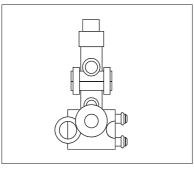
The pneumatic control blocks are used to activate the consumers (bottom valves). The pre-control block is generally used to activate the vent valves. The visual display on the control block indicates the activated consumers.
